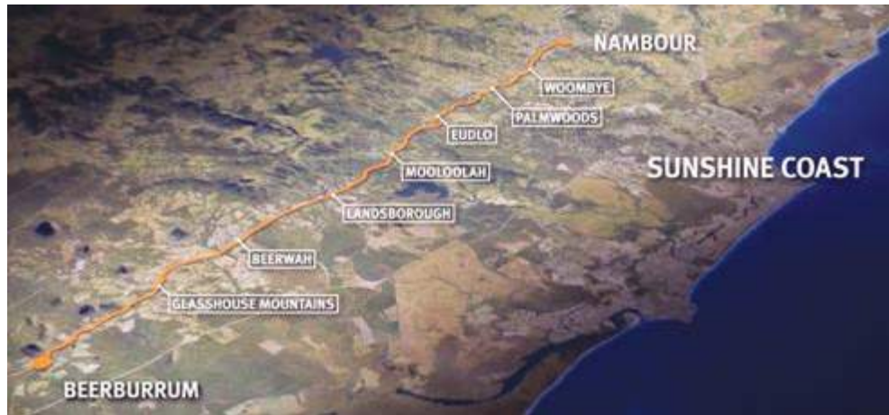
The 39km section between Beerburum and Nambour is currently a single track with trains using passing loops at stations to pass each other.
